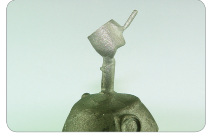
3) Body completed via centrifugal casting machine
