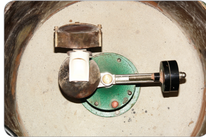
2) Centrifugal casting machine used commonly for casting
