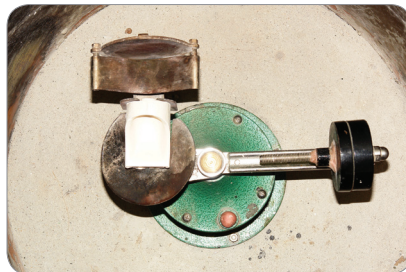
2) Centrifugal casting machine used commonly for casting
